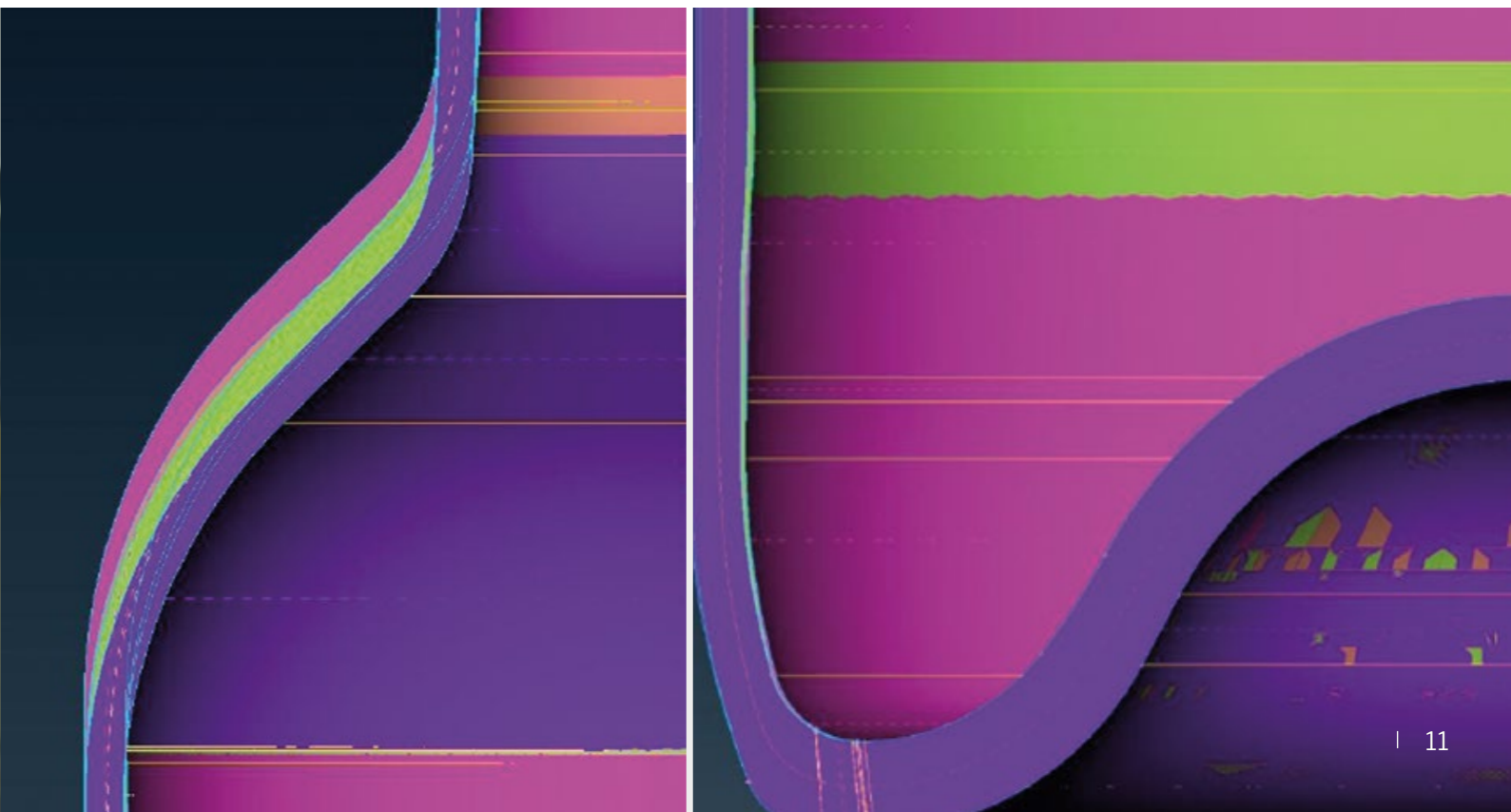
Glass thickness correlation: glass bottle vs. simulations.
