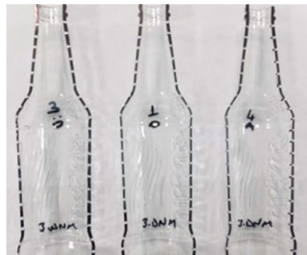
Bottle cut analysis after sampling.
