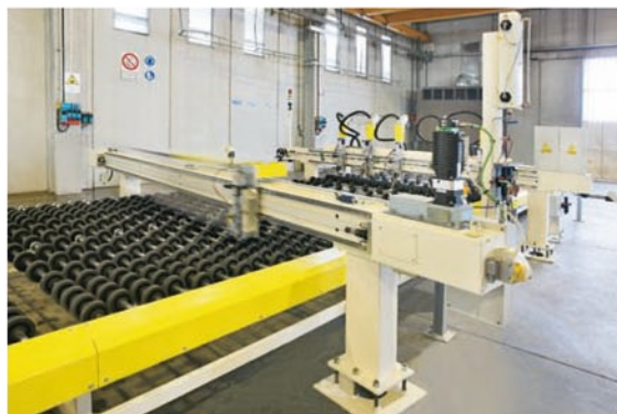
Patterned cutting bridge.
